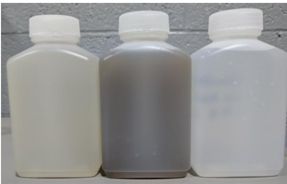
Raw wastewater, TSRO concentrate, and TSRO permeate (clean water)
