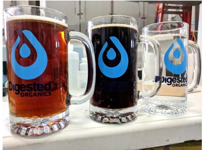
Ultrafiltered dairy manure, stack concentrate, and TSRO permeate (clean water)
