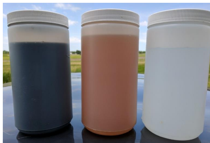
Wastewater, UF Permeate, and TSRO Permeate
